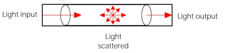
2. The interaction of the electromagnetic field of the light with the material waves in the fiber ("Brillouin")
