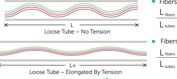
EFL = Excess Fiber Length = the "extra" fiber per unit length of tube or cable (from stranding) General Rule: Higher is better ("No strain = No problem")
