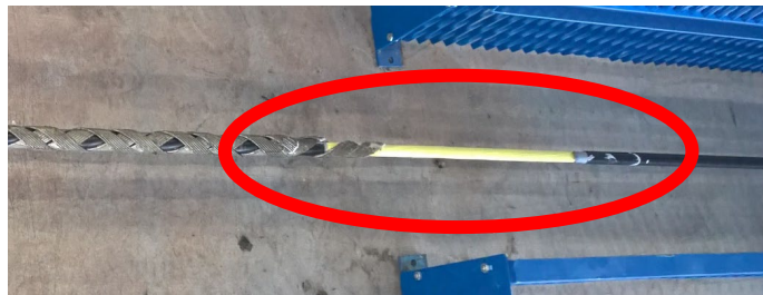
A jacket tear in a lab on a known de-coupled ADSS cable design
