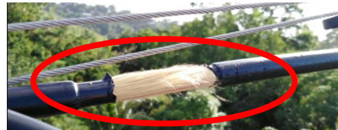
A jacket tear in the field on an ADSS cable believed to be de-coupled design
