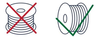
When arranging multiple reels of the same size, ensure that the flanges of each reel face each other. Compressing the cable between adjacent reels may cause damage.
