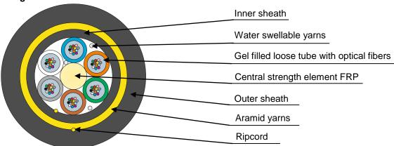
Cable consists of stranded core with central strength element (FRP), gel filled loose tubes with optical fibers. Stranded core is fixed by water swellable yarns. Inner sheath is made of LDPE. Aramid yarns are laid over inner sheath. Outer sheath is made of MDPE. One ripcord is laid under each sheath. Meets IEEE 1222-2011.
