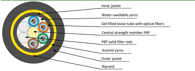
Cable consists of stranded core with central strength member (FRP), gel-filled loose tubes with optical fibers and PBT solid filler rods (natural color). Stranded core is fixed by water-swellable yarns. Inner jacket is made of LDPE. One ripcord is laid under inner jacket. Aramid yarns are laid over inner jacket. Outer jacket is made of MDPE. Two ripcords are laid under outer jacket. Meets IEEE 1222-2011.
