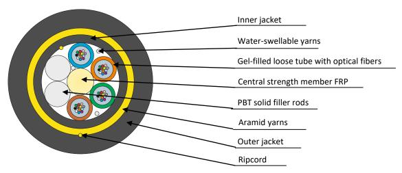
Cable consists of stranded core with central strength member (FRP), gel-filled loose tubes with optical fibers and PBT solid filler rods (natural color). Stranded core is fixed by water-swellable yarns. Inner jacket is made of LDPE. Aramid yarns are laid over inner jacket. Outer jacket is made of MDPE. One ripcord is laid under each jacket. Meets IEEE 1222-2011.
