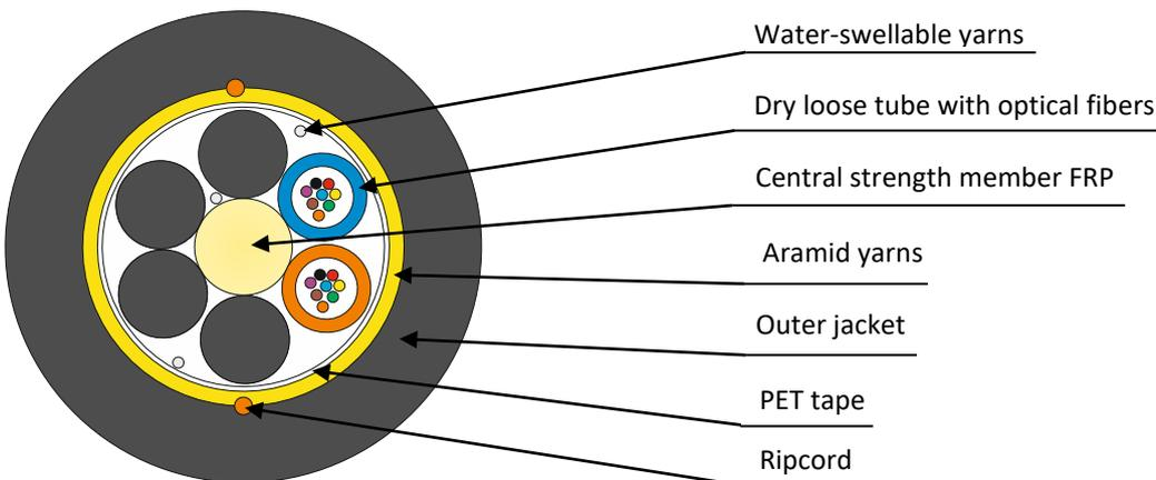
Cable consists of stranded core with central strength member (FRP), dry loose tubes with optical fibers and PE fillers (black color). PET tape is laid over loose tubes layer. Stranded core is fixed by water-swellable yarns. Aramid yarns are laid over stranded core. Outer jacket is made of MDPE. Two ripcords are laid under outer jacket.
