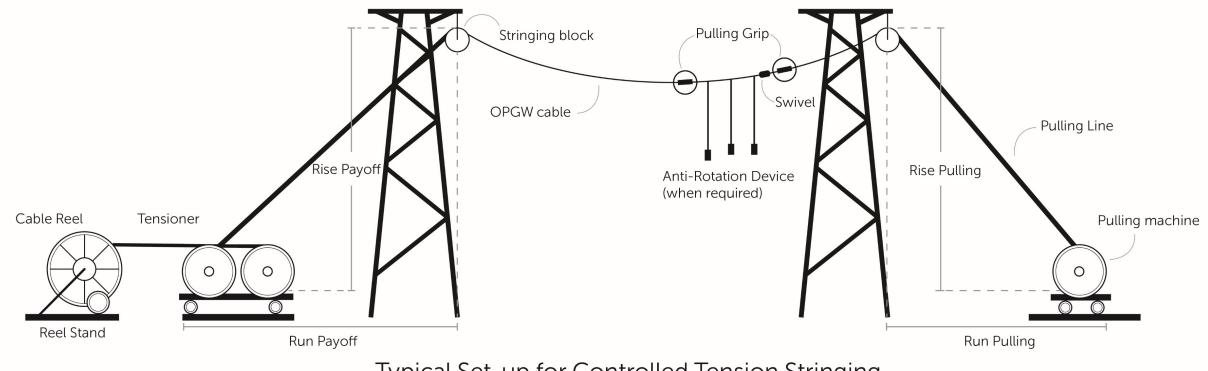
Typical Set-up for Controlled Tension Stringing
