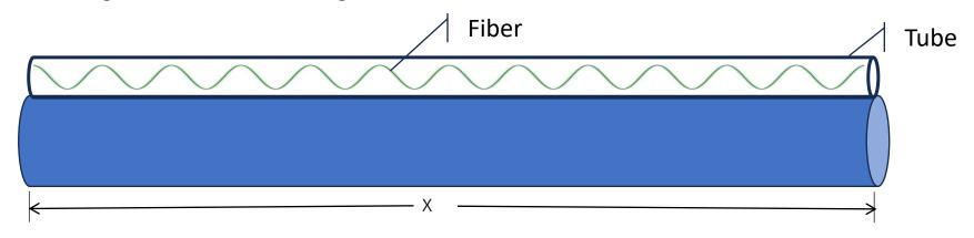
That is: L <sub>fiber</sub> > L <sub>tube</sub>
