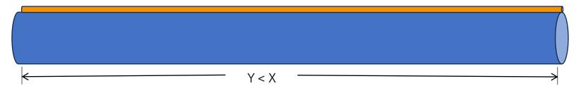
A higher temperature or increased wind or ice loading will cause the cable and fiber to stretch:
