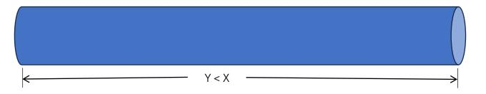
• A higher temperature or increased wind or ice loading will cause the cable to stretch:
